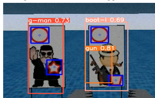
Figure 2.9 Identifying and classifying the targets in torpedo task
